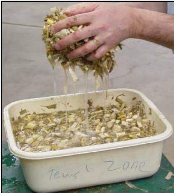
Figure 3. Skimming and removing the floating stover.
