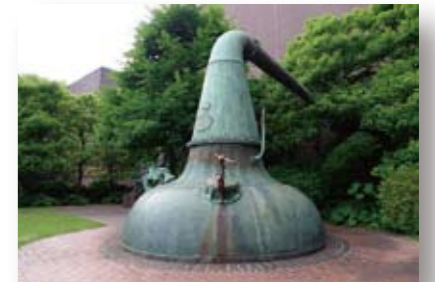
Pot still (single distillation still) used to manufacture Japan's first whisky in 1923.
